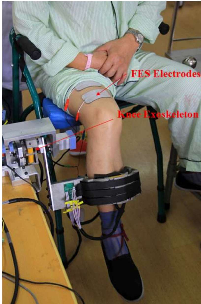
Figure 20. Experimental set up of hybrid FES-exoskeleton rehabilitation system.
