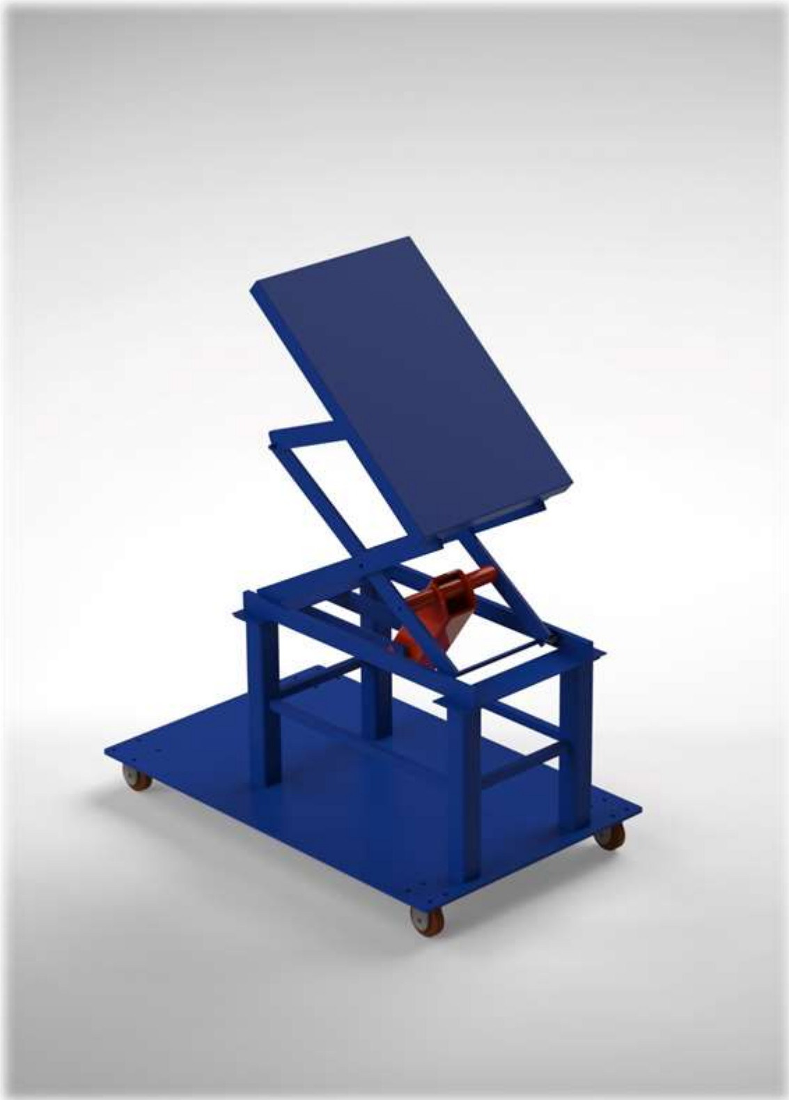
Figure 5. Scissor Lift-frame of 3rd generation RWTD.
