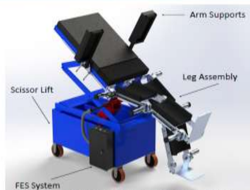
Figure 1. RWTD showing the 4 main components of the project.
